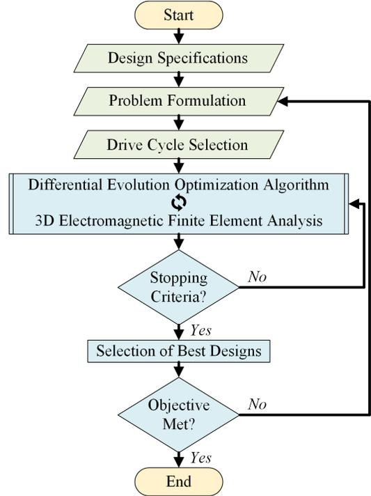
Fig. 11. The flowchart of the proposed optimization process using differential evolution algorithm combined with the single-point drive cycle analysis.
