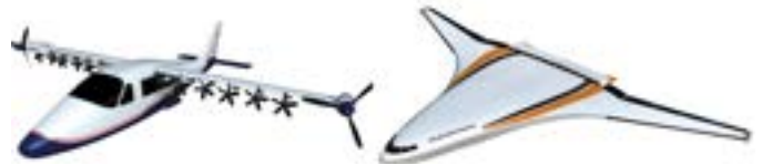
Figure 1. Example distributed electric propulsion aircraft designs by NASA with varying power system topologies. All-electric demonstrator X-57 Maxwell currently under development utilizing multiple electrical machines with varying ratings [2] (left). Conceptual turbo-electric N3-X aircraft which utilizing electrical energy from generators coupled to jet engines [3] (right).
