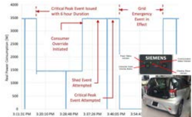
Fig. 1. The performance test results for CTA-2045 EV supply equipment published by Electric Power Research Institute (EPRI) [5]. Shown are the EV for testing, visual indicators and controls on electric vehicle service equipment EVSE, and results for different control signals.
