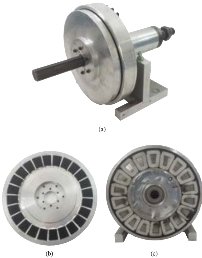
Fig. 15: The motor designed for the vehicle application and experimental validation: (a) the assembled machine, (b) the rotor, (c) the stator.
