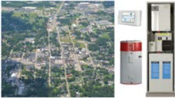
Fig. 1. Aerial view of Glasgow, KY, the location of the studied SET, along with pictures of smart devices for home energy management: thermostat, EWH and BESS, which are programmable and enabled by WiFi or Ethernet. The data acquired has a resolution of up to 1 minute and is available for both home owners and the utility.
