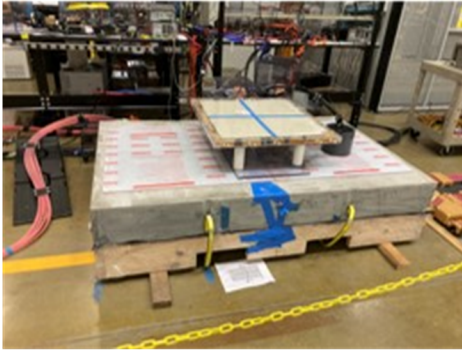
Fig. 1. A prototype transmitter and receiver coil pair for wireless charging testing and a diagram of an example wireless power transfer system for charging electric vehicles with power-systems level control and power electronics control to compensate for variability. Models employed in this study are based on previously published prototypes from ORNL experimentally validated at 85kHz, 120kW operation and simulated up to 200kW [1].
