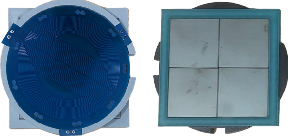
Fig. 7. Prototype DD PCB coil at 100 mm OD with ferrite core backing. PCBs allow for many turns with increased customization and manufacturability at smaller ODs through special design techniques.
