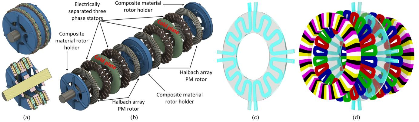
Figure 1. Proposed coreless AFPM machine with an integrated cryogenically cooled thermal management system, illustrating (a) compact and sectional views of the double-stage design, (b) the exploded view of the full assembly, (c) the topology of the cold plate positioned between the two stators in each module, and (d) the exploded view of a single stage.
