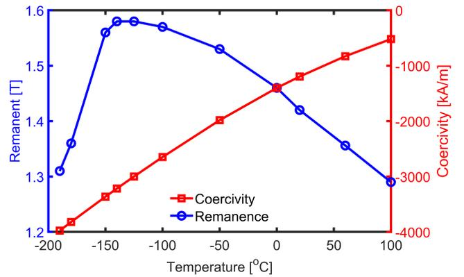
Figure 2. Remanence and coercivity curves of NdFeB 50BH at various temperatures.
