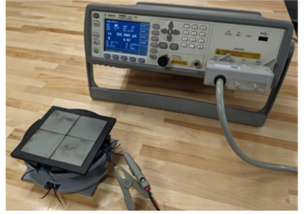
Fig. 9. Experimental setup for the measurement of inductances between the primary and secondary coils with a three to two phase 100mm OD PCB prototype.
