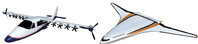
Figure 1. Example distributed electric propulsion aircraft designs by NASA with varying power system topologies. All-electric demonstrator X-57 Maxwell currently under development utilizing multiple electrical machines with varying ratings [2] (left). Conceptual turbo-electric N3-X aircraft which utilizing electrical energy from generators coupled to jet engines [3] (right).
