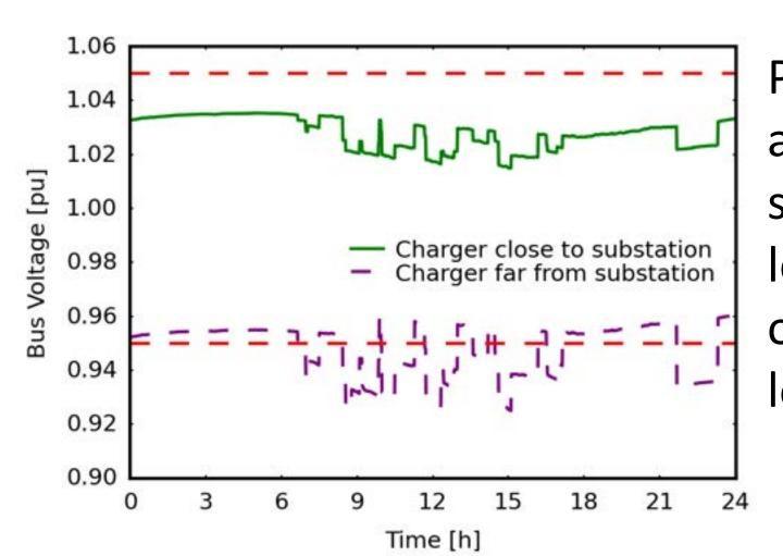
Point of interconnection further the substation from shows violation of voltage lower limit for high utilization of 50kW charger, which is the lowest assessed
