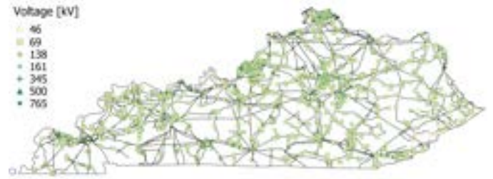
Fig. 10. Transmission lines and substations according to the US HIFLD [24] are located in high density in the areas of renewable potential, specifically in central and northern parts. Further considerations of line and substation ratings, capacity, and location are needed to support studies for a future smart grid with 100% DER generation.
