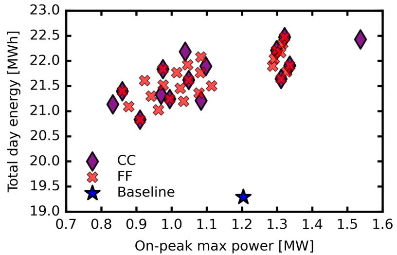
**Fig. 8.** Resulting evaluation of optimization objectives for both the central composite (CC) and full factorial (FF) design of experiments (DOEs) with respect to the baseline case. The VPP controls are capable of reducing the maximum peak power as shown by the CC and FF results to the left of the baseline case, indicating that an optimization to select the control windows is justified and would be beneficial.
