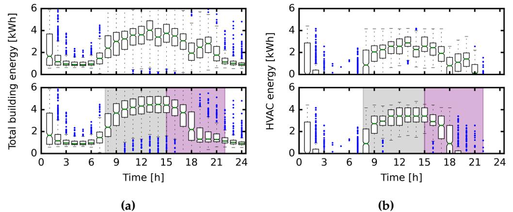
**Fig. 12.** Results for individual building (a) total energy use and (b) HVAC energy use only of the baseline and P6 cases.
