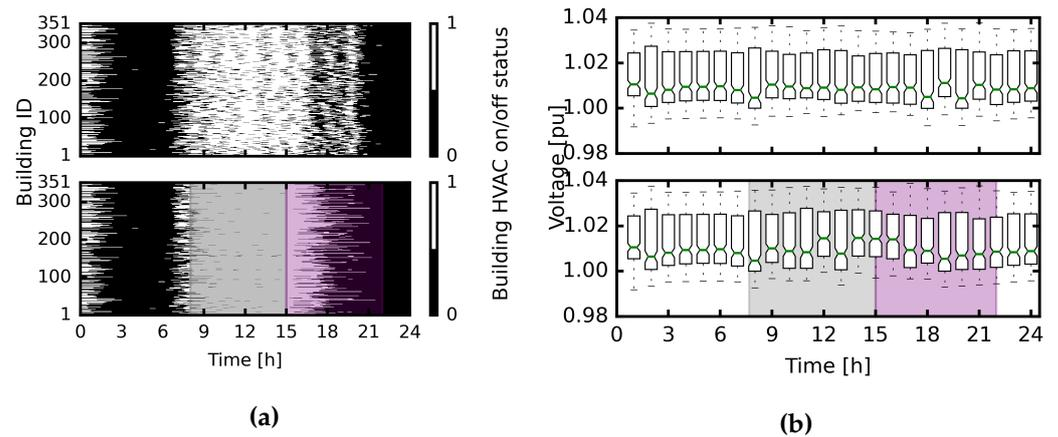
**Fig. 7.** Simulation results for **(a)** individual on/off statuses for HVACs to show control phasing in the baseline case (top) and in case P6 (bottom) as well as **(b)** hourly average bus voltages for both the baseline and P6 cases. The “load-up” and “shed” event windows are shaded in light gray and purple, respectively. This format is replicated in following figures.
