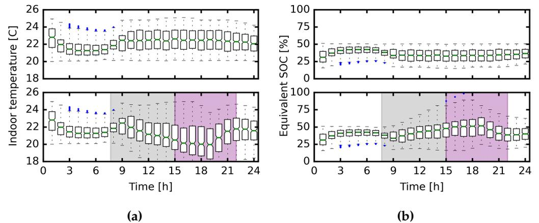
**Fig. 13.** Hourly average (a) indoor temperatures and (b) equivalent SOC, which is inversely related to indoor temperature, of all buildings for the baseline and P6 cases.
