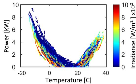
**Fig. 3.** Example HVAC “V-curve” and physical relationship between weather parameters and power captured by the ML model. In principle, the ML model may be applied with weather at different locations and employ the approximately linear trends to estimate the power demand.
