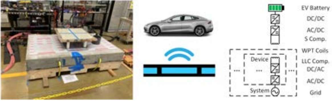
Fig. 1. A prototype transmitter and receiver coil pair for wireless charging testing and a diagram of an example wireless power transfer system for charging electric vehicles with power-systems level control and power electronics control to compensate for variability. Models employed in this study are based on previously published prototypes from ORNL experimentally validated at 85kHz, 120kW operation and simulated up to 200kW [1].
