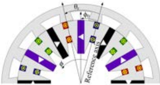
Fig. 3. Cross-section of a half periodicity region for the proposed motor design with 7 rotor protrusions. The noted angular coordinates as indicated are used in the analysis of the machine. The reference axis is middle of the stator slots.
