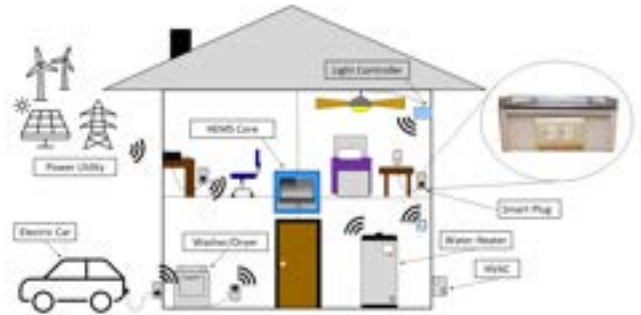
Figure 3. An HEMS controls manage smart appliances in the home to respond to user and utility controls. Intrusive load monitoring (ILM) devices, such as the illustrated smart plug [17], are monitoring equipment for advanced appliance level controls.
