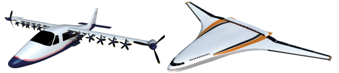
Figure 1. Example distributed electric propulsion aircraft designs by NASA with varying power system topologies. All-electric demonstrator X-57 Maxwell currently under development utilizing multiple electrical machines with varying ratings [14] (left). Conceptual turbo-electric N3-X aircraft which utilizes electrical energy from generators coupled to jet engines [15] (right).
