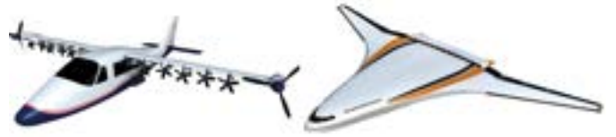
Figure 1. Example distributed electric propulsion aircraft designs by NASA with varying power system topologies. All-electric demonstrator X-57 Maxwell currently under development utilizing multiple electrical machines with varying ratings [14] (left). Conceptual turbo-electric N3-X aircraft which utilizes electrical energy from generators coupled to jet engines [15] (right).
