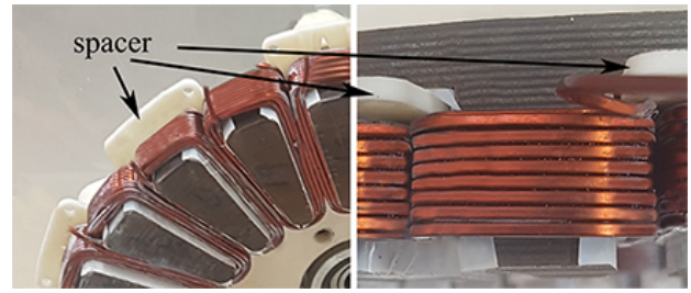
Fig. 4: The prototype machine with spacers.
