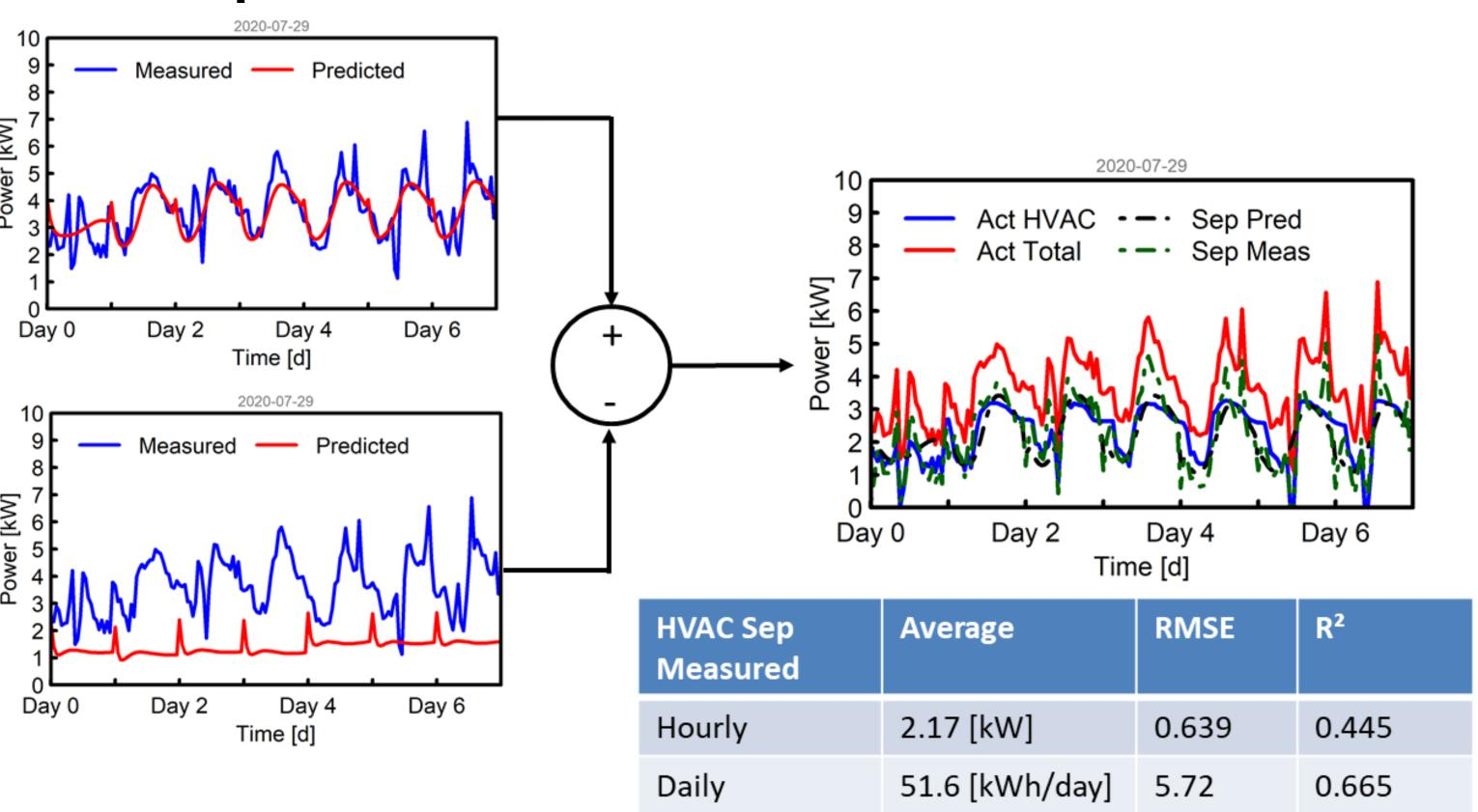
A method to separate the HVAC load from total smart meter data:
