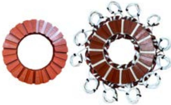
Fig. 10: The prototyped profiled stator core and active stator wound with coils.
