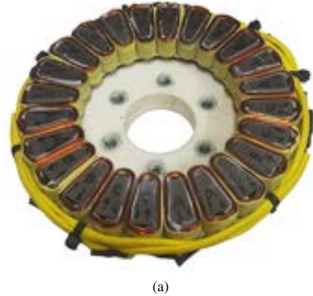
Fig. 15. The optimum designs obtained for the configuration with 30 poles. (a) The design with minimum loss on the Pareto front, (b) the design with minimum cost on the Pareto front, (c) the design on the knee of the Pareto front with a trade-off between cost and loss.
