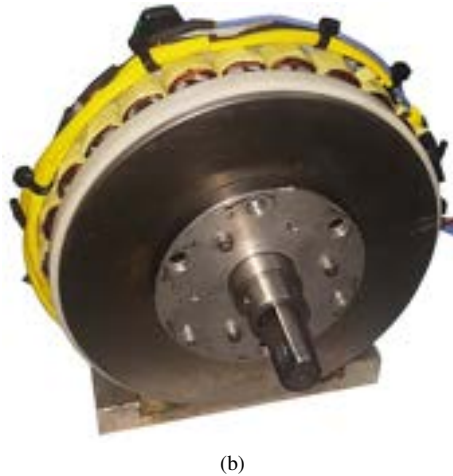
Fig. 17. The ultra high efficiency AFPM machine, rated for 5.4 Nm at 1050 rpm, selected for prototyping based on the comprehensive optimization study with 3D FEA models. (a) The stator with a core OD of approx. 170 mm and (b) the assembled motor.
