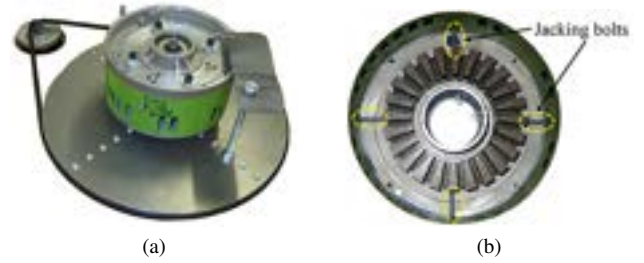
Figure 2. (a) Fractional hp AFPM motor and special experimental set-up for varying static eccentricity and measuring cogging torque. (b) Four jacking bolts at 90 degree intervals are used to adjust the eccentricity by manipulating the stator position.
