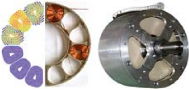
Figure 20. Special concentrated-winding multi-disk laboratory prototype employed for validating the 3D FEA parametric design study. The detailed fine finite element mesh and current density vectors in the coils calculated from 3D FEA are represented on the left.
