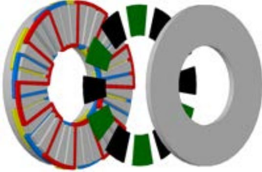
Figure 2. Exploded view of the 3D model of the NGM SC-M150 motor with 36 stator slots and 12 rotor poles.
