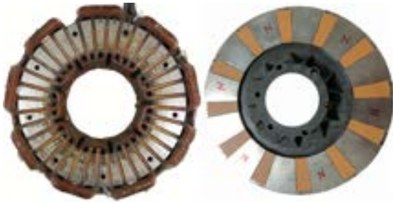
Figure 3. The stator of the NGM SC-M150 motor installed in Gato del Sol IV solar car together with a new prototype rotor.
