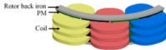
Fig. 2: Two pole pairs of the 3D model with surface mounted PMs.
