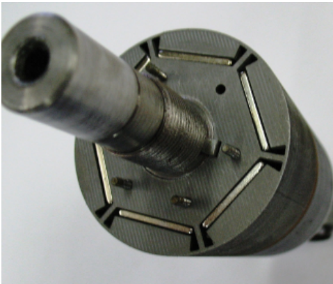
Fig. 3. The rotor of the example prototype motor considered in the study.
