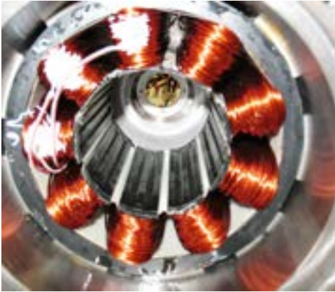
Fig. 2. The stator of the example prototype motor considered in the study.
