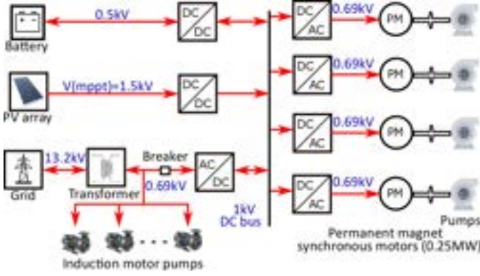
Fig. 1. Schematic overview for the expansion of an existing grid-connected irrigation pumping system with the addition of solar PV, battery, and PMSM inverter driven pumps for capacity modulation.
