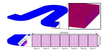
Fig. 8. Meshing of the detailed 3D model for the wave winding PCB stator and a cross section illustration of traces within the macro coil.
