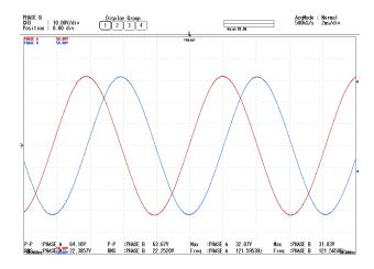
the two phases. The experimental results for one phase of the two phase AFPM machine closely matches the OC back-EMF of the trace-by-trace model as shown in Fig. 14.
