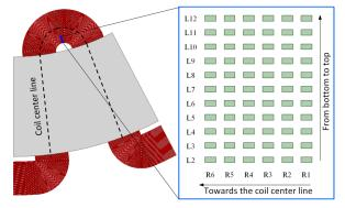
Fig. 9. Cross section of a single turn (Turn 7) of the wave winding PCB stator with 12 vertical layers and 6 columns.
