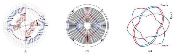
Fig. 1. Typical PCB winding configurations, (a) distributed winding (one phase shown), (b) spiral winding, (c) progressive wave winding (two coil units are shown for phase A and one coil unit is shown for phases B and C). The spiral winding and continuous wave winding are inherently suitable for high-polarity designs.
