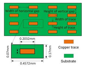
Fig. 3. Cross section of a PCB coil example. There are 16 traces equally spaced in the substrate. Only the envelope geometry, i.e., the macro coil, is modeled in the 3D FEA and trace information is reflected in the fill factor.
