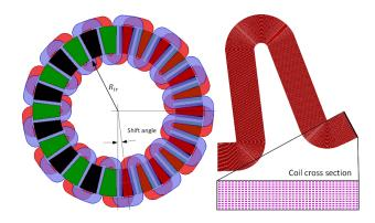
Fig. 2. Coreless AFPM machine with a wave winding PCB stator. A 2-phase PCB stator is illustrated as an example with two PCBs stacked onto each other and shifted by 90 elec. degrees.
